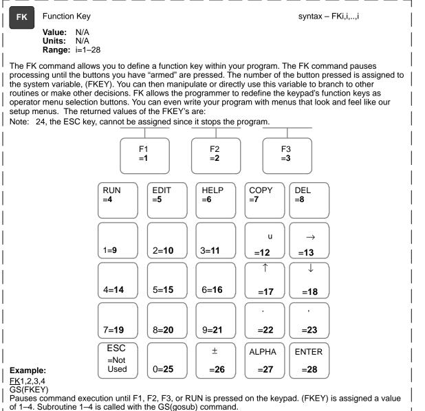
Figure 6-1 shows how to use the keypad function keys as an operator interface. A 3–screen menu program is provided
